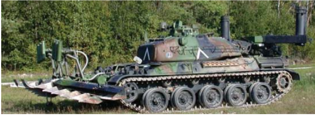
Fig. 4. Remotely controlled French tank (AMX30B2) for mine clearance operations
