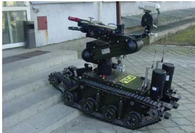
Fig. 3. The first dedicated IED disposal robotic platform "Wheelbarrow"
